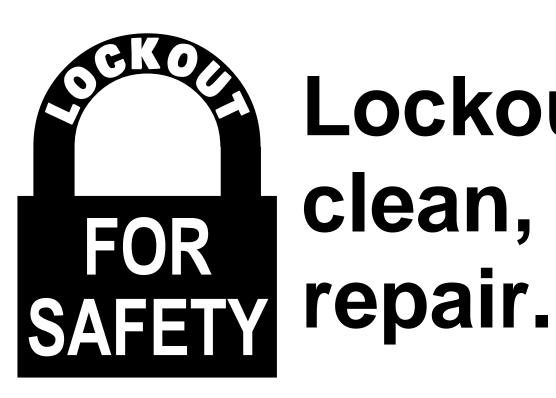
Lockout power to clean, oil or repair.
